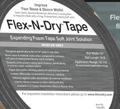
Flex-N-Dry<sup>™</sup> Tape is a UV stable, pre-compressed, self-expanding, flexible, flame-resistant soft joint alternative. It is a high-density polyurethane foam impregnated with a modified acrylic resin and treated with a pressure-sensitive adhesive on one side for ease of installation. Flex-N-Dry Tape self-expands to fill a <sup>3</sup>/<sub>8</sub>"-<sup>5</sup>/<sub>8</sub>" joint creating an elastic, vapor-permeable and weather-tight seal.
